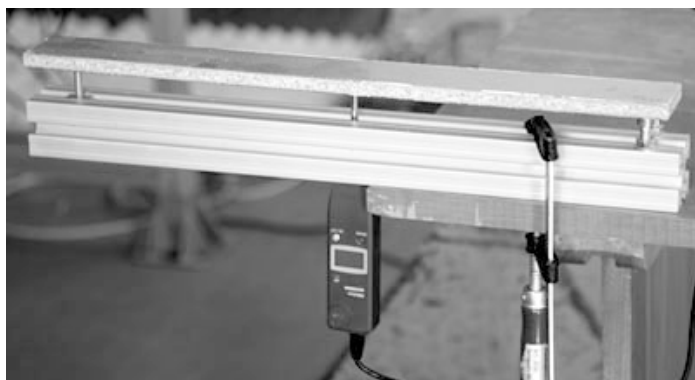
Fig. 2. A sample's deflection measurement
